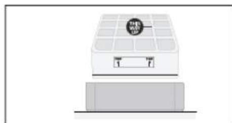
9. Turn the frame over (right side up again) and insert the new filter. Ensure that the arrows on the filter label point upward.
