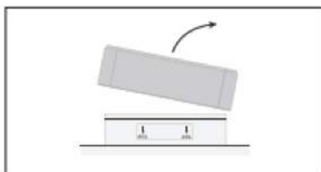
8. Dispose of the used filter by placing it into the plastic bag in which the new filter is supplied (see section 6.7).
