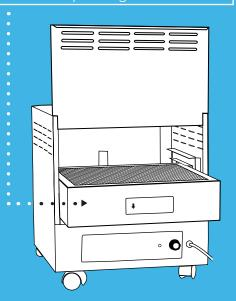
STEP 1: Make sure Mobile System is unplugged and slide up the back panel to remove
