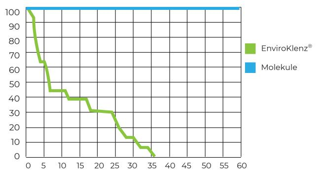
In the third graph (located above), the two devices were challenged with NH3. Over the course of the 60-minute test, the EnviroKlenz system was able to completely neutralize the chemical compounds, while the Molekule had no detectable impact on the concentration of the compound in the air.
