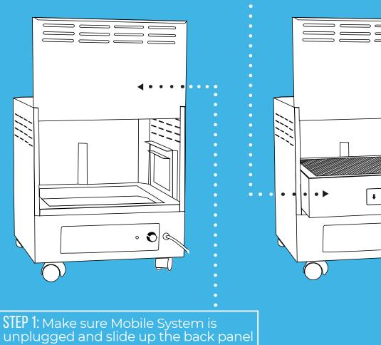
STEP 2: Slide in larger HEPA Filter with airflow arrow pointing down
