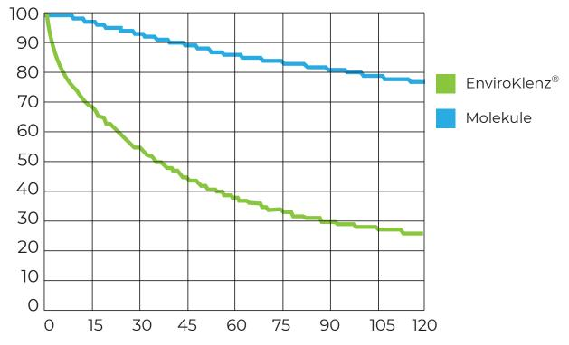
In the second graph (located above), the two devices were challenged with formaldehyde, a common indoor air pollutant. The target starting ppm range for these tests was 6 ppm. The EnviroKlenz<sup>®</sup> Air System steadily reduced the concentration by 50% in 45 minutes, while the Molekule only achieved around a 20% reduction at 2 hours.
