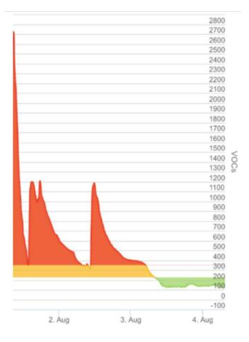
The same study was conducted the following week, and the results were the same. As illustrated in the image to the left, the VOC levels before the EnviroKlenz<sup>®</sup> Mobile Air System deployment spiked during the daytime production hours, while they remained relatively stable after the system was deployed.
