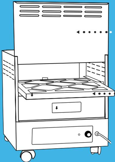
**STEP 4:** Replace sliding back panel with blank side facing out
