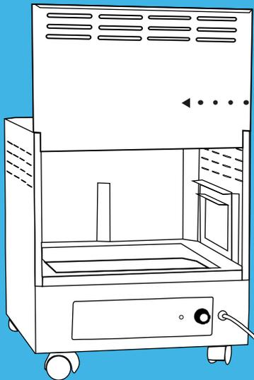
STEP 1: Make sure Mobile System is unplugged and slide up the back panel to remove
